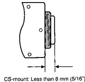
**Caution:** To use the C-mount lens, the Lens Mount Converter (C-mount adapter) WV-AD20 should be used with the camera.
