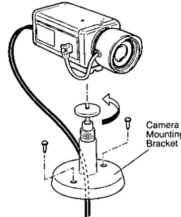
**Note:** Coaxial cable can be passed through the center hole of the camera mounting bracket.
